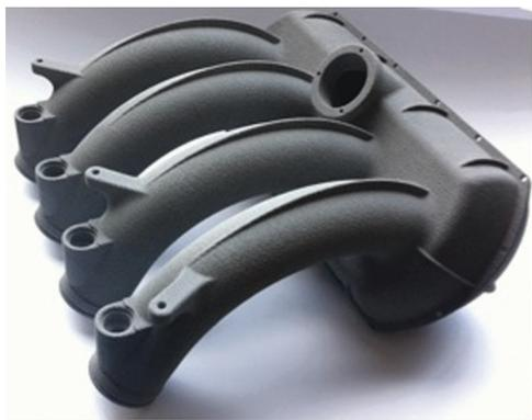
**Fig. 32** Specific part manufactured by selective laser sintering directly to its final shape, using a blend of polymer and icosahedral AlCuFeB. This part is ready for sale and is an example of a successful, marketed application of quasicrystals.<sup>51</sup>
