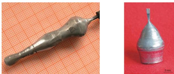
**Fig. 17**  $\text{Al}_4(\text{Cr,Fe})$  (left) and  $\text{Al}_{13}\text{Co}_4$  (right) single grain crystals grown out of Al-rich liquids. Courtesy of P. Gille, University of Munich.
