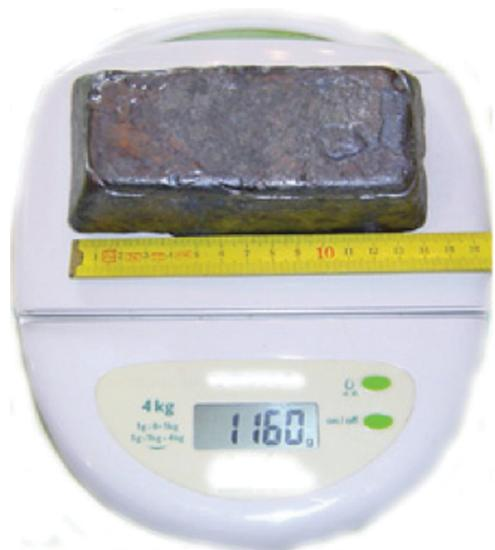
**Fig. 15** Photograph of an Al–Cu–Fe–Cr ingot (weight: 1.16 kg) produced in large quantities to prepare atomized powders for plasma spray of approximant coatings on frying pans. The capability was set to 1000 kg per day.<sup>31</sup>
