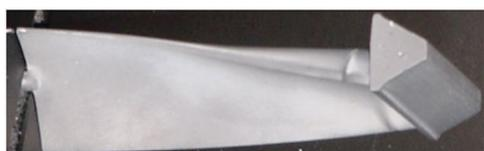
Fig. 26 Small turbine blade covered with a 0.3 mm thick thermal barrier made by magnetron sputtering of an AlCoFeCr CMA (the length of the blade is typically 8 cm). This application fits the needs of helicopter engines, which work at moderate temperatures of the order of 700 °C. Courtesy of S. Drawin, ONERA.
